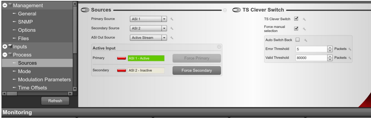
Figure 5: TS manual switching
